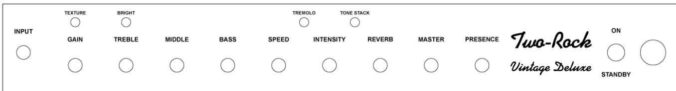
**INPUT** - High impedance input to the amplifier. Plug in your instrument here.
