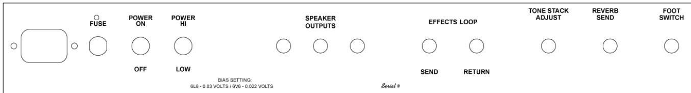
**A/C Input** - Connects the amplifier to A/C power via the power cable supplied. Unless otherwise specified, your amplifier is designed to operate on 120 volts A/C, 60 cycles.
