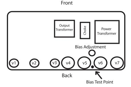
Each fine production tube is tested and matched to our exacting specifications. External bias adjustment and test points are located on the chassis near the output tube sockets. A digital voltmeter and small screwdriver are required for bias adjustment.
