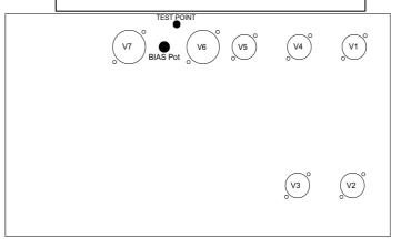
Each fine production tube is tested and matched to our exacting specifications. When the time comes that the power tubes need replacing, it's very important to use high quality, matched sets of power tubes. It's also critical that the bias of the amp be reset after installing new, or NOS power tubes. External bias adjustment and test points are located on the bottom of the chassis near the output tube sockets. A digital voltmeter and small screwdriver are required for bias adjustment.
