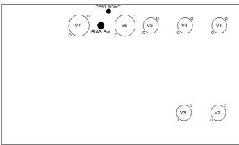
V1 - 12AX7 - Input and Gain V2 - 12AX7 - Reverb Send & Return V3 - 12AT7 - Reverb Drive V4 - 12AX7 - Effects buffer & Mixing Stage V5 - 12AX7 - Phase Inverter V6-V7 - 6L6
