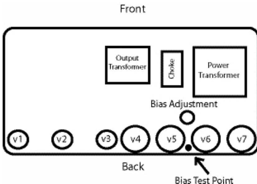
Each fine production tube is tested and matched to our exacting specifications. External bias adjustment and test points are located on the chassis near the output tube sockets. A digital voltmeter and small screwdriver are required for bias adjustment.
