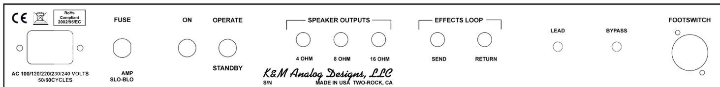
**A/C Input-** Connects the amplifier to A/C power via the power cord supplied. Unless otherwise specified, your amplifier is designed to operate on 120 volts A/C, 60 cycles.
