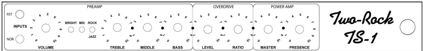
**NOR Input Jack**- High impedance input to the amplifier. Plug in your instrument here.
