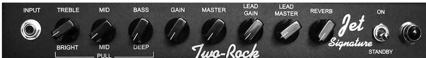
**Input Jack-** High impedance input to the amplifier. Plug in your instrument here.
