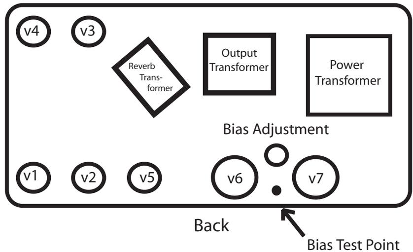
Each fine production tube is tested and matched to our exacting specifications. External bias adjustment and test points are located on the chassis near the output tube sockets. A digital voltmeter and small screwdriver are required for bias adjustment.
