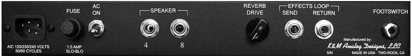
**A/C Input-** Connects the amplifier to A/C power via the power cord supplied. Unless otherwise specified, your amplifier is designed to operate on 120 volts A/C, 60 cycles, ONLY!
