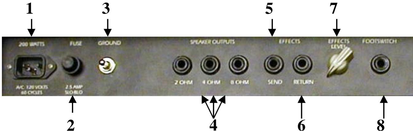
1. **A/C INPUT-** Connects the amplifier to A/C power via the power cord supplied. Unless otherwise specified, your amplifier is designed to operate on 120 volts A/C, 60 cycles.
