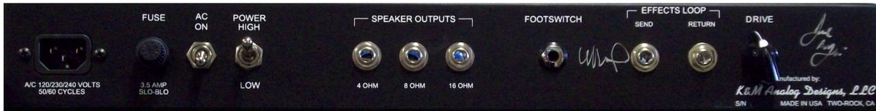
1. **A/C Input-** Connects the amplifier to A/C power via the power cord supplied. Unless otherwise specified, your amplifier is designed to operate on 120 volts A/C, 60 cycles.
