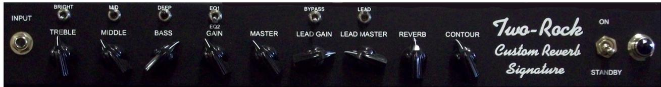
1. **Input Jack**- High impedance input to the amplifier. Plug in your instrument here.
