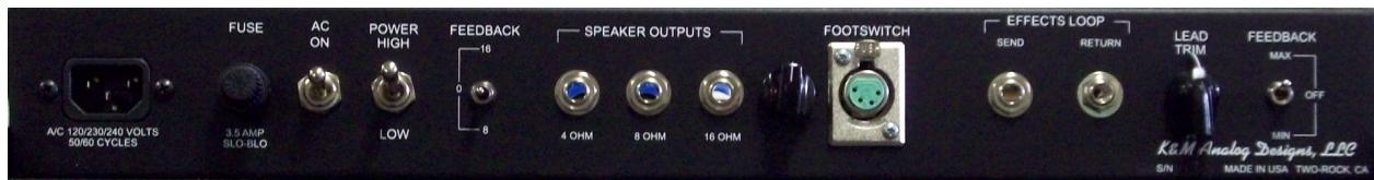
**A/C Input-** Connects the amplifier to A/C power via the power cord supplied. Unless otherwise specified, your amplifier is designed to operate on 120 volts A/C, 60 cycles, ONLY.
